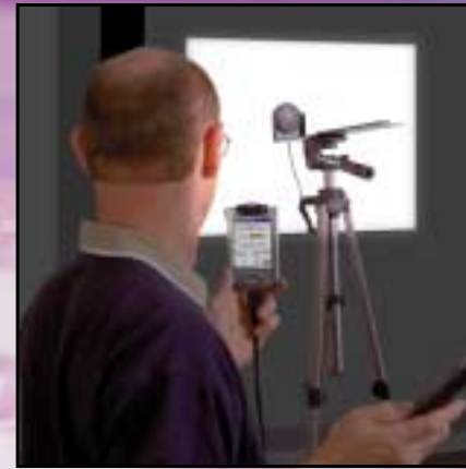
A calibrationist uses a color analyzer to adjust background color.
